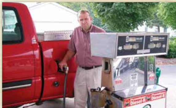
Figure 3.1 Fatty Acid Methyl Esters can be used in existing equipment without modification due to the physical and chemical changes that occur during transesterification of vegetable oil.
