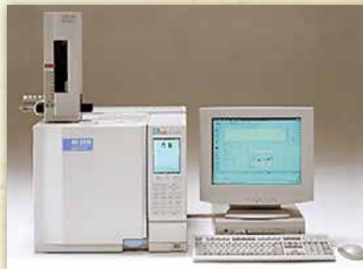
Figure 4.1 A Gas Chromatograph allows scientists to examine complex mixtures of chemicals accurately. Photo courtesy of Shimadzu Inc.
